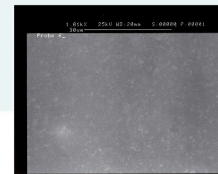
SEM* image of a standard ventricular catheter, typically of silicone
